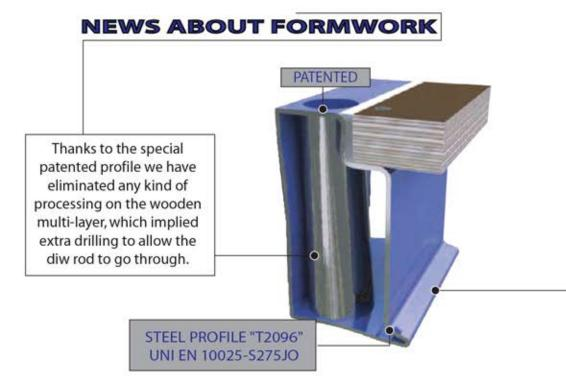
With this kind of innovation, the passage of the bar takes place only on the inside of the profile, thus allowing a longer duration to the multi-layer, which does not have critical points for water absorption anymore. Moreover, it is characterized by an indispensable protruding edge on the lower part, which enables our alligner clamp to assemble formworks in a linear and precise way .-
